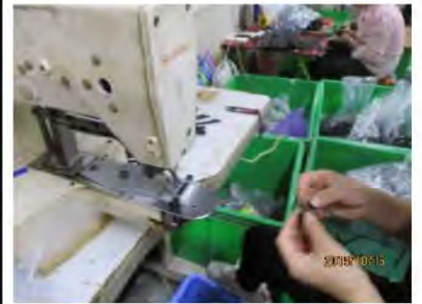
27. NC-No safety eye-shield was installed
